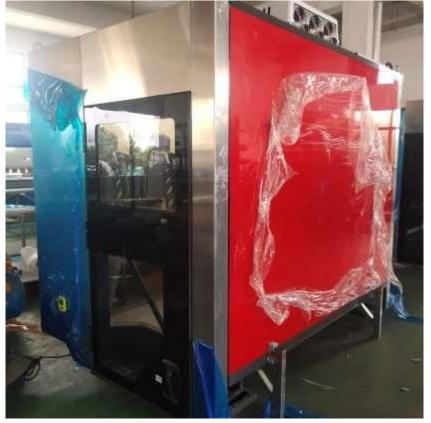
The top plate, bottom plate, and front and rear sealing plates are made of specialized non-metallic composite honeycomb panels, which have good insulation and sound insulation properties;
