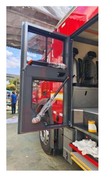
All glass door panel structure, with good light transmittance and field of view;
