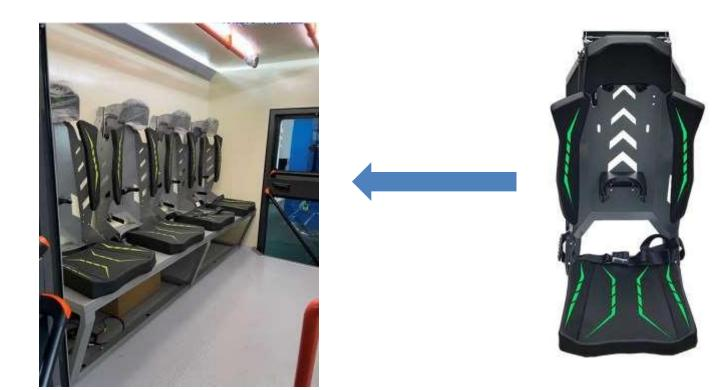
Firefighters' dedicated seats with seat cushion flipping or seat cushion fixation can be configured according to requirements
